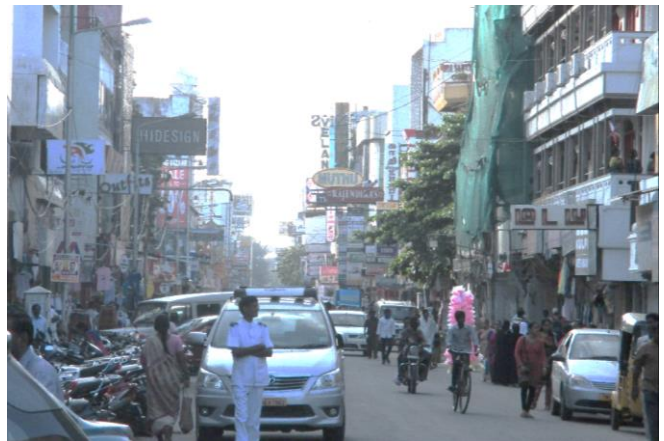
Figure 5-22 JN Street – On street parking reducing the effective width of the carriageway
